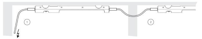
This illustration shows the LED 025 lamp in a daisy chain application. The lamps are conveniently connected via quick connection plugs – up to 10 lamps max. can be daisy-chained this way. The snap lock connectors ensure a stable electrical connection even if subjected to heavy vibration. The connection example shows a 230VAC application, using the following cables: connection cable with female connector, Art. No. 244356 (1); daisy chain extension cable with 2 connectors, Art. No. 244358 (2).
